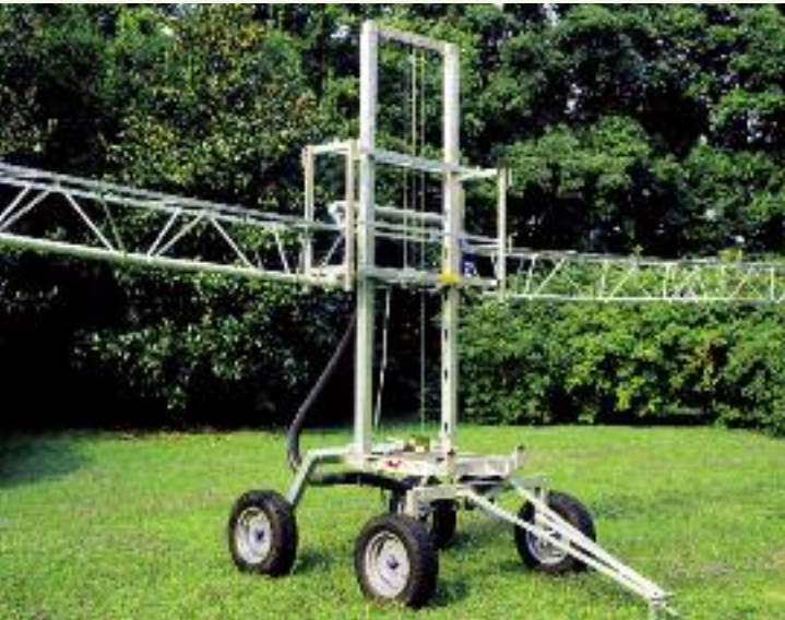
carrello porta ala a 4 ruote variabile in altezza con verricello - chariot porte-rampe a 4 roues, variable en hauteur, avec treuil - carretilla porta ala de 4 ruedas variable en alto con chigre - 4-wheels trolley with height adjustment by means of a winch.
